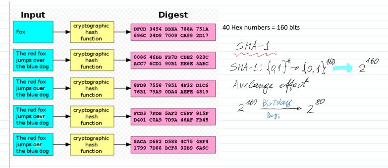
A cryptographic hash function (specifically <u>SHA-1</u>) at work. A small change in the input (in the word "over") drastically changes the output (digest). This is the so-called avalanche effect.
